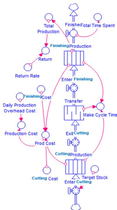
Figure 2. DES Model of The Table Production
