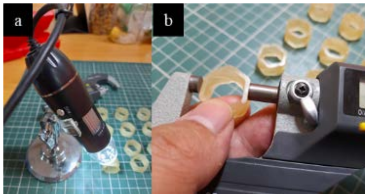
Figure 2. The 3D printed models observed by a digital microscope (a) and measured by a digital micro calliper
