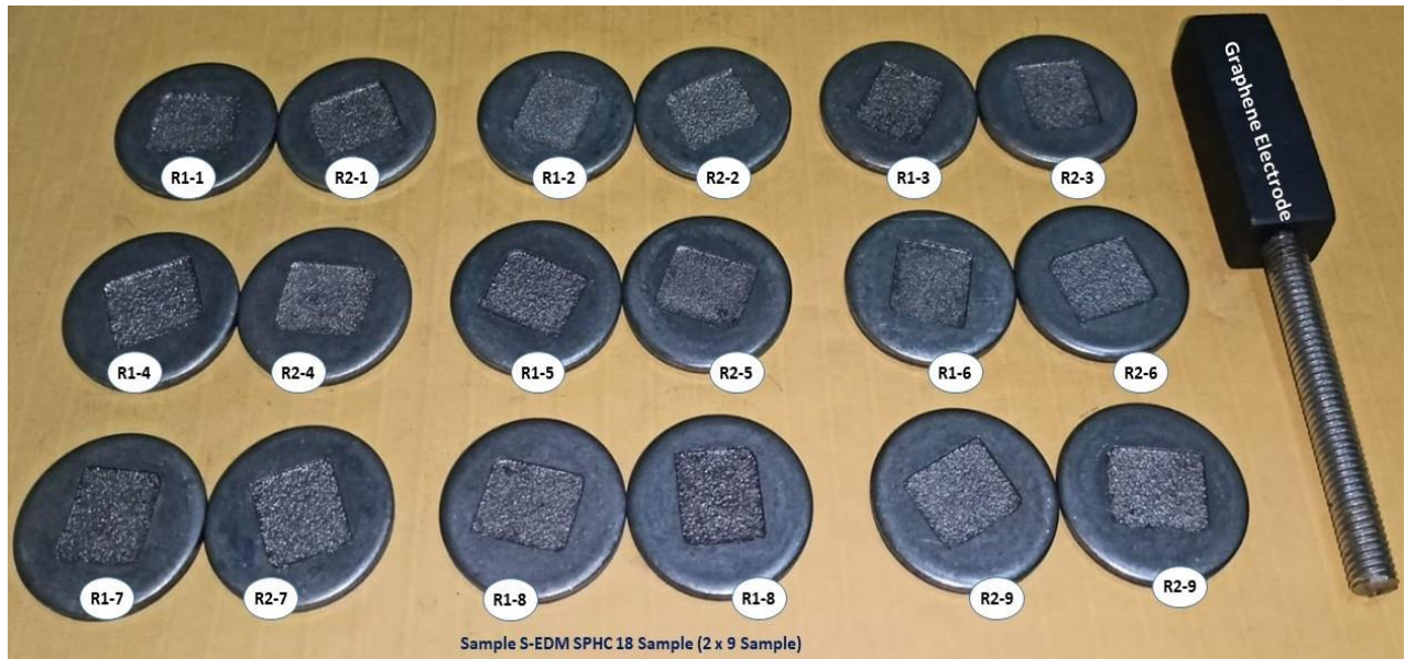
Figure 2. The sinker EDM sample of SPHC work material and graphene electrode
