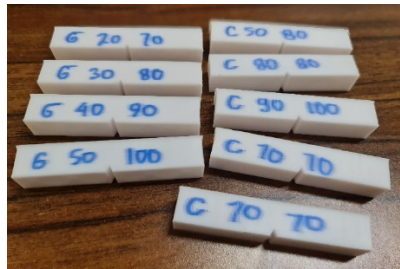
Figure 3. The specimens are ready for Charpy impact testing
